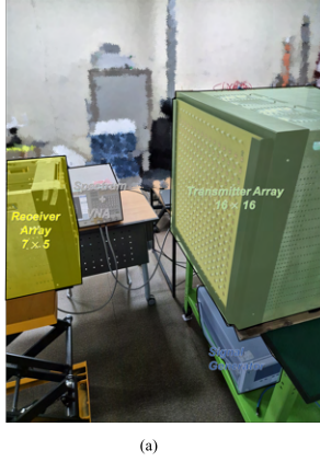
Fig. 7. (a) The measurement environment and the results of the received RF power for (b) ideal condition and (c) measurement at 0.5 m distance.
