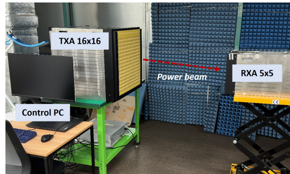
Fig. 6. Hardware setup for DC-to-DC optimization validation.
